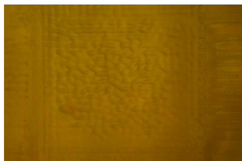
Figure S2. Optical micrograph of printing artifacts on plastic (PET) confirming that printing artifacts are independent of substrate (7 layers of PVP, 718cP).
